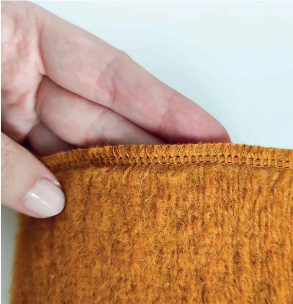
6. Once the sleeves are installed and garment is right side-in, pin front and back pieces on both sides, making sure that armhole seams are matched. Sew both sides with 4-thread overlock seam. iron the seams.
