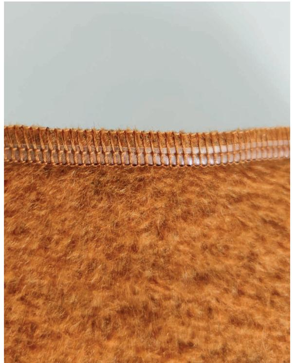
Here is how a 4-thread overlock seam looks with stabilizing silicone strap:
